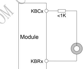
Figure 40: Enhance the ESD performance of keypad circuit
