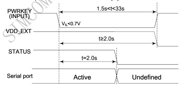
Figure 14: Timing of power off SIM808 by PWRKEY
