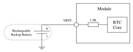
Figure 20: RTC supply from rechargeable battery
