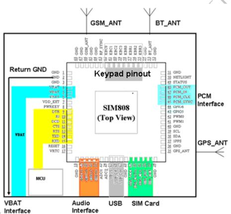
Figure 50: PCB layout pinout example
