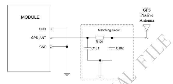
Figure 48: GNSS passive antenna matching circuit
