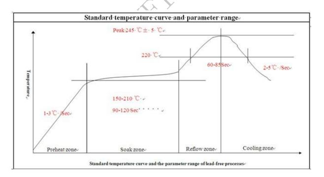
Figure 52: Typical Solder Reflow Profile
