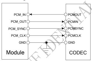
Figure 38: PCM reference circuit
