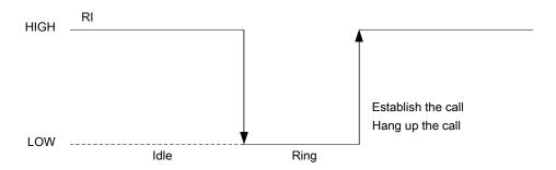
Figure 28: RI behaviour of data calling as a receiver
