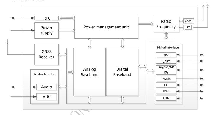
Figure 1: SIM808 functional diagram
