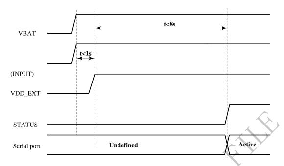
Figure 13: Timing of power on module
