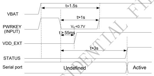
Figure 12: Timing of power on module
