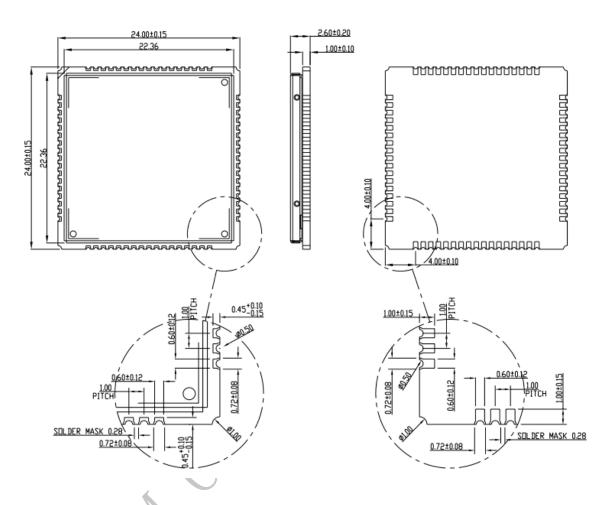
Figure 3: Dimensions of SIM808 (Unit: mm)
