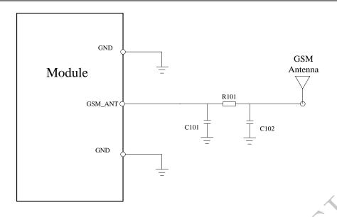
Figure 46: GSM simple antenna matching circuit
