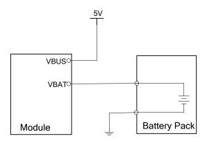
Figure 17: SIM808 with battery charger and pack connection
