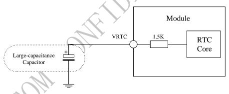
Figure 18: RTC supply from capacitor
