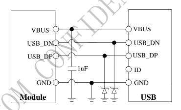
Figure 26: USB reference circuit
