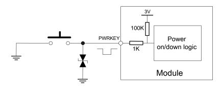
Figure 11:Powered on/down module using button
