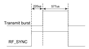
Figure 44: RF\_SYNC signal during transmit burst
