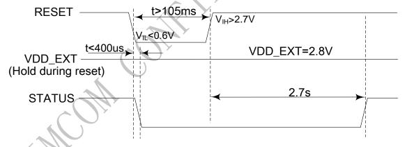
Figure 16: Reset timing sequence
