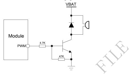
Figure 42: Reference circuit of PWM drive buzzer
