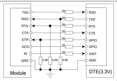
Figure 22: Level converting by resistor
