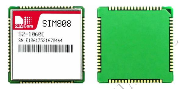
Figure 51: Top and Bottom View of SIM808
