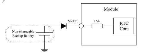
Figure 19: RTC supply from non-chargeable battery
