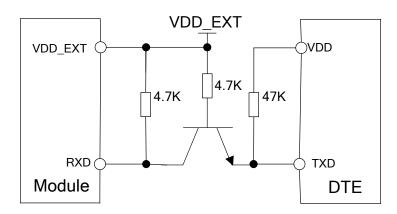
Figure 25: RX level converting by transistor
