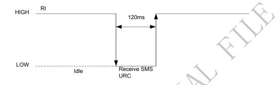
Figure 29: RI behaviour of URC or receive SMS
