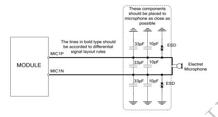
Figure 33: Microphone reference circuit
