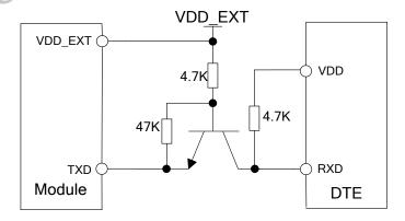
Figure 24: TX level converting by transistor
