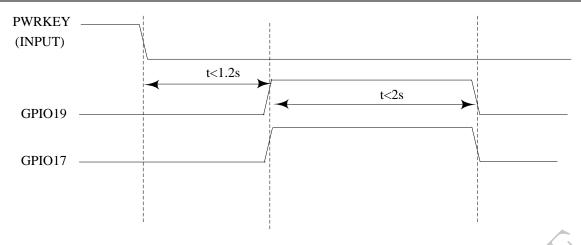
Figure 41: GPIO timing sequences
