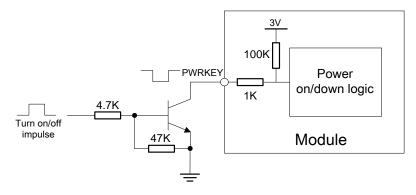
Figure 10: Powered on/down module using transistor
