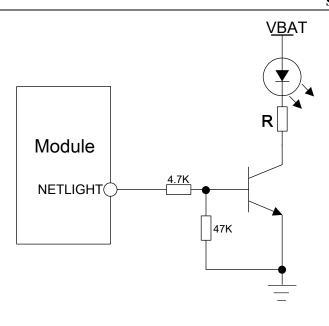
Figure 43: Reference circuit of NETLIGHT
