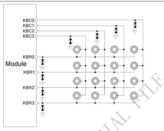
Figure 39: Traditional keypad reference circuit
